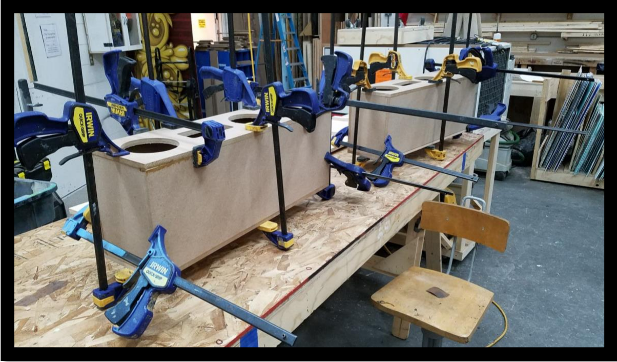
MDF interior boxes glued & clamped
