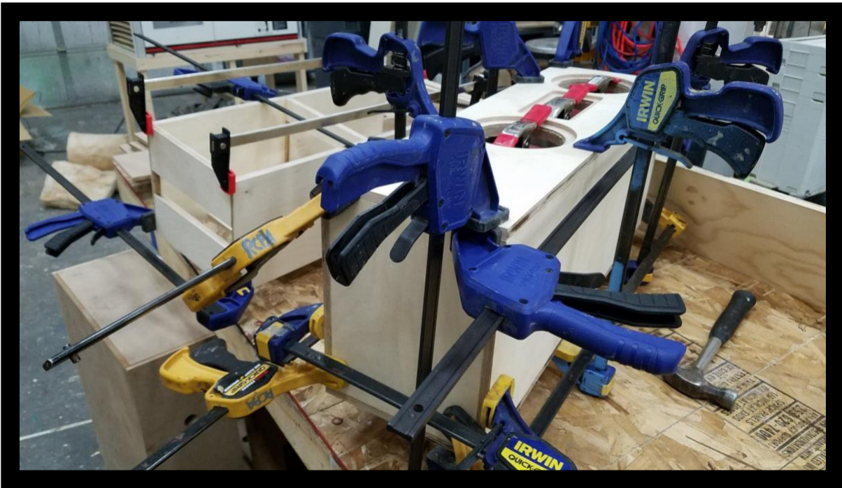
Exterior Baltic Birch layers glued & clamped along with Baltic Birch loudspeaker stand clamped
