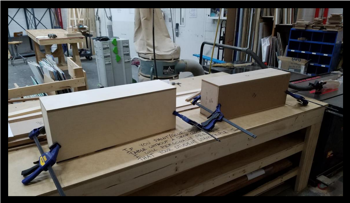
Plywood & MDF boxes assembled separately to check for any mis-cuts
