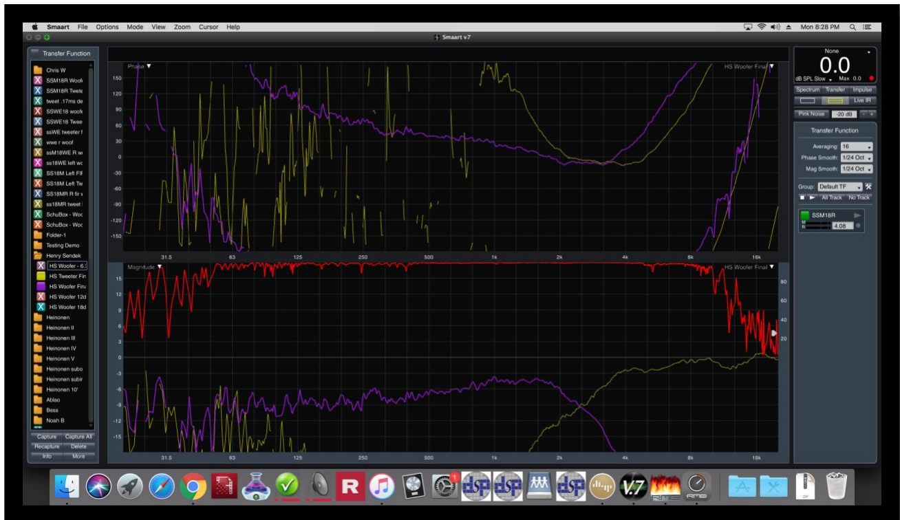
SMAART: Phase Alignment between Woofers & Tweeter
