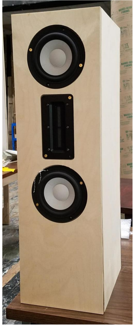
The above picture on the left is my fully constructed enclosure immediately after the box was finished gluing The above picture on the right is the same enclosure after installing my drivers in their test positions
