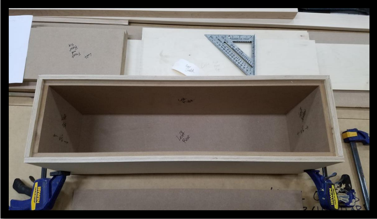
Plywood & MDF boxes assembled together to check for any size issues
