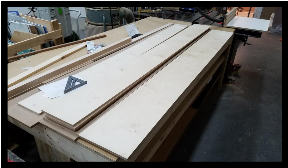
MDF & Plywood 4'x8' sheets after being run through the table saw
