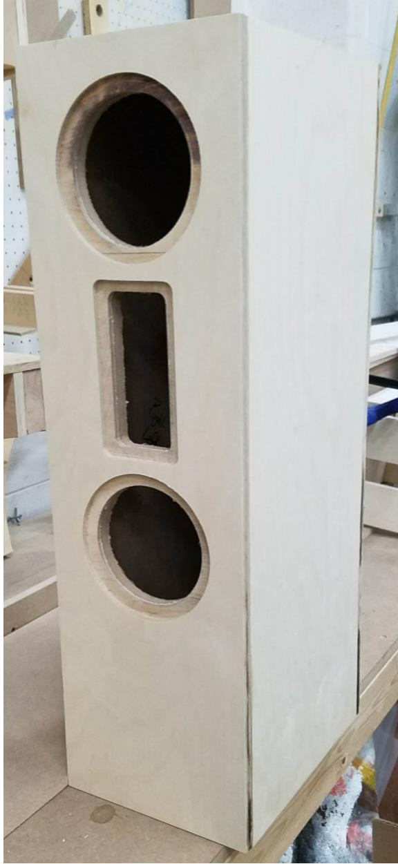
The above picture on the left is my fully constructed enclosure immediately after the box was finished gluing The above picture on the right is the same enclosure after installing my drivers in their test positions
